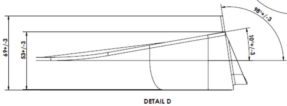
FrontSplitterBrackets' design is free however the front splitter must be rigidly fixed the car's body at least in the area between the vertical projection of the front side members. Outside this area flexible front splitter mountings are allowed. (Certification)
